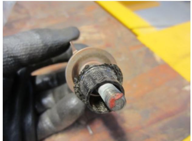
Picture 22: Worn stg.5 bushing example
