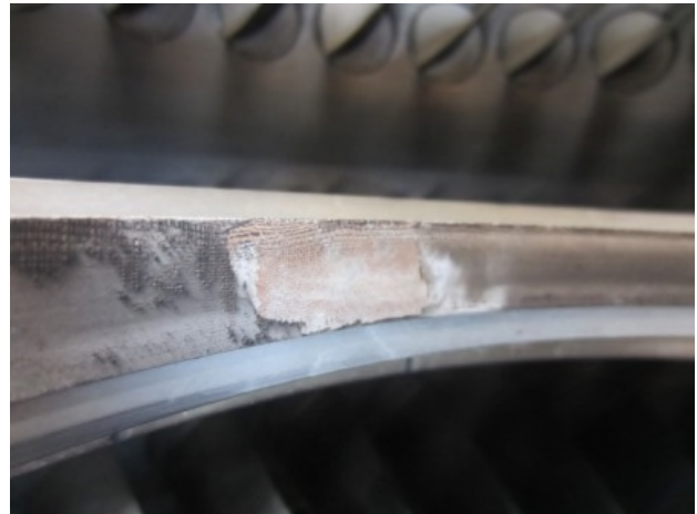
Picture 20: Spalled coating on stg.1 shroud
