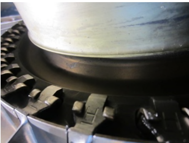
Picture 17: Bended stage 1 blade retainers
