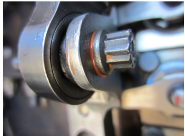
Picture 28: Red silicone in stg.5 link as support
