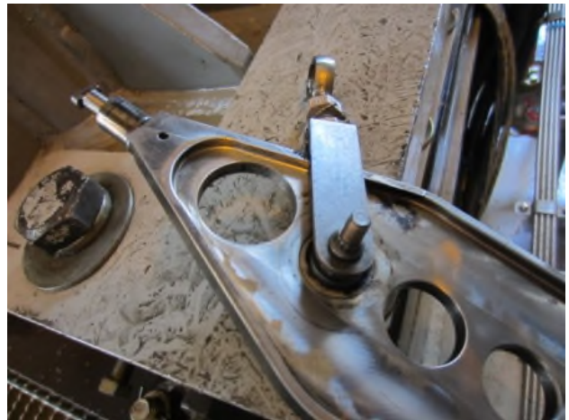
Picture 4: L/H stg. IGV clevis with missing boot
