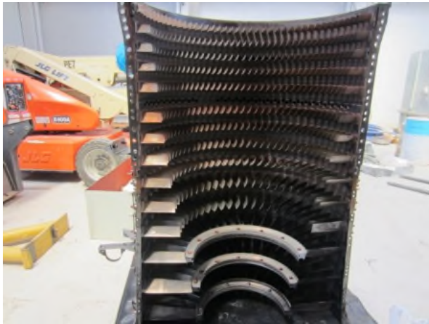
Picture 19: Upper stator case in workshop
