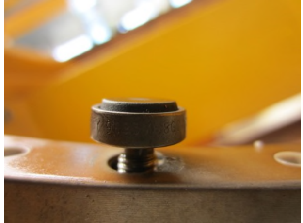
Picture 26: New actuating ring spacer installed
