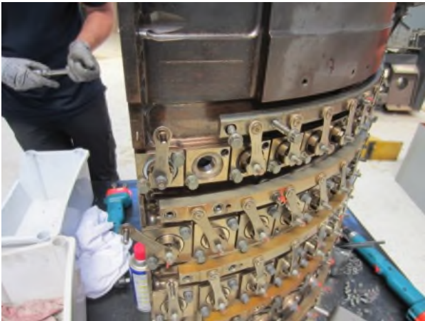
Picture 21: Washer / bushing replacement upper case
