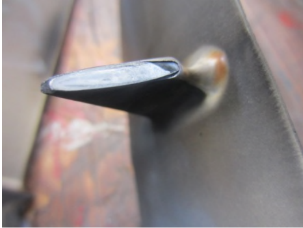
Picture 13: Old mid span damper pad stage 1
