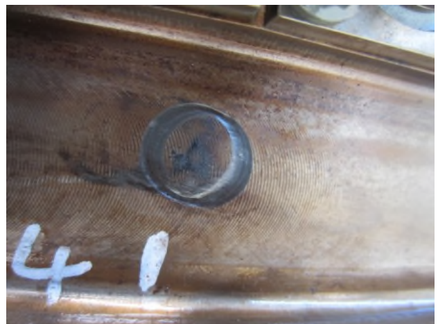
Picture 24: Chafing marks on stage 4 stator case
