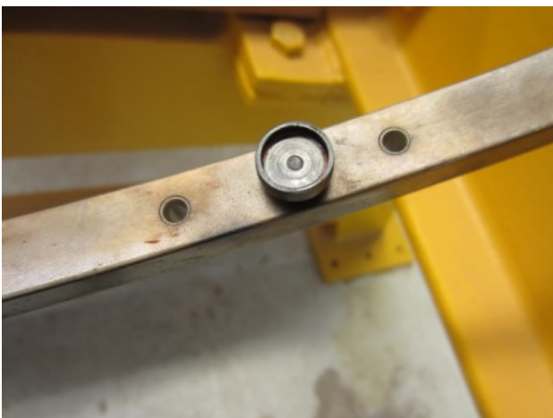
Picture 23: Missing insert in actuating ring spacer
