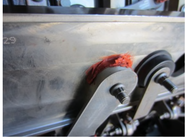
Picture 2: Stage 5 clevis with red silicone
