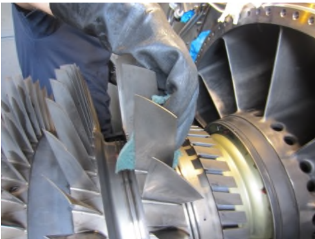
Picture 15: Hand cleaning of hpc blades
