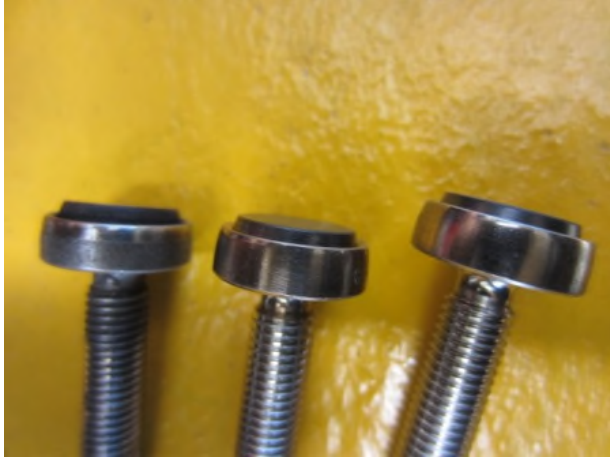
Picture 25: New actuating ring spacer with inserts
