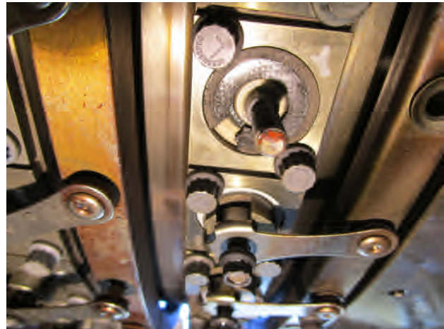
Picture 10: missing washer material stage 5
