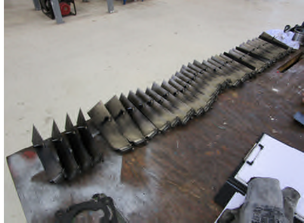
Picture 14: removed stage 1 blade set (36 ea)
