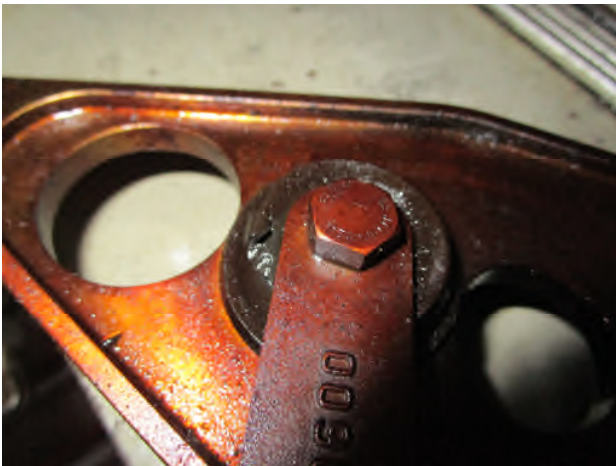
Picture 5: Viton boot left hand side with crack
